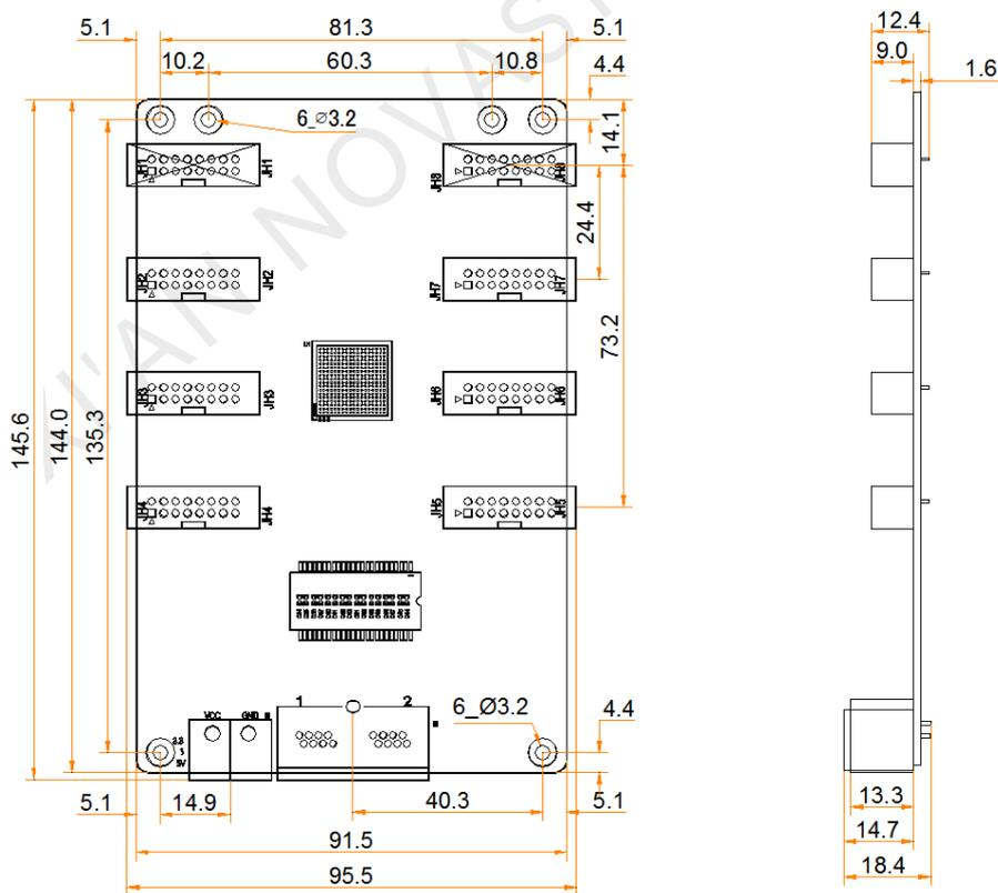
Tolerance: ±0.3 Unit: mm
